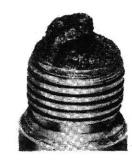
IDENTIFIED BY WET BLACK DEPOSITS ON THE INSULATOR SHELL BORE ELECTRODES.
